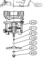
(5) Remove the casing cover (011) from the motor base (044), and pull out the sleeve (031), sleeve packing (032), mechanical cover (340), and deflector (250) from the motor shaft (681).
