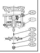
(031), sleeve packing (032), Remove the casing cover (011) from the motor base (044), and pull out the sleeve (031), sleeve packing (032), mechanical cover (340), and deflector (250) from the motor shaft (681).
