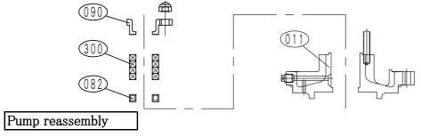
Reassembly of the pump is possible by the reverse order of disassembly.
