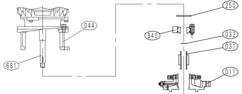
\* For mechanical sealing pump, loosen the set screw and pull out the mechanical seal rotating ring (310) from the sleeve (031).
