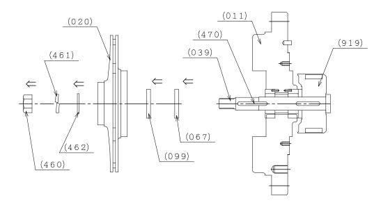
5. Remove the bolow shaft (039) with the inner drive (919) from the casing cover (011). Take out the metal (069) from the casing cover (011). Remove the set pin (065).
