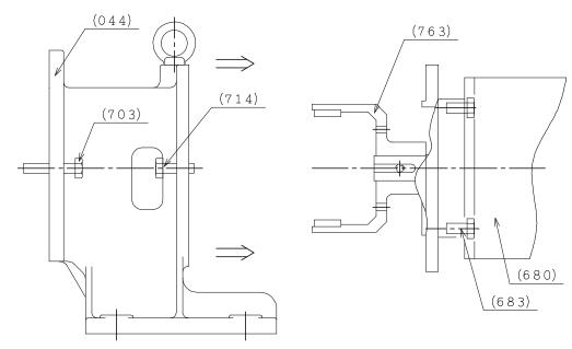
[Exercise caution with the magnets inside the couplings, during a drive coupling and motor removal.]
