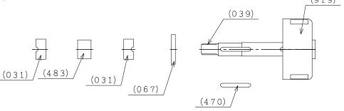
8. Remove the inner drive (919) from the bolow shaft (039), and then remove the inner drive key (474).
