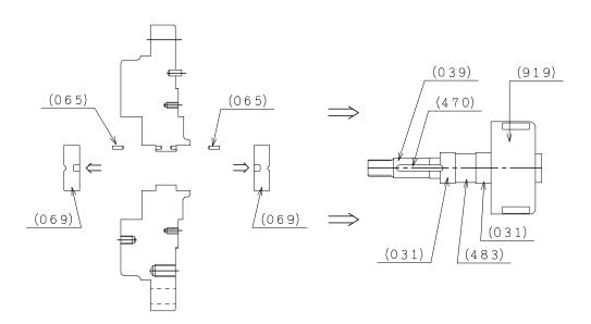
6. Remove the impeller key (470) from the bolow shaft (039).
